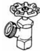
Boiler Valve Figure 4
